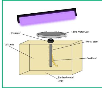
A gold leaf electroscope, with a zinc metal cap, is given a charge at the beginning of an experiment. This causes the gold leaf to rise.
