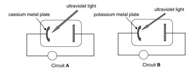
Ultraviolet light with the same intensity and wavelength of  $5,5 \times 10^{-7}$  m is incident on the metal plate in EACH of the photocells and the ammeter in circuit **A** registers a current.
