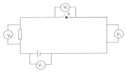
Which voltmeter reading is INCORRECT when the switch is opened, as shown?
