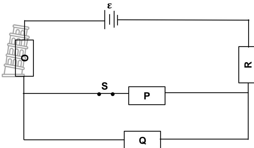
Switch **S** is now OPENED. Which ONE of the following combinations of changes will occur in **O**, **Q** and **R**?
