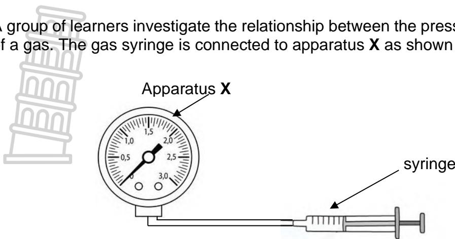
The learners vary the volume and record the pressure and volume. They calculated the inverse of the volume and recorded it with the pressure readings in table shown below.
