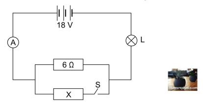
Switch S is OPEN and the ammeter reads 2 A.
