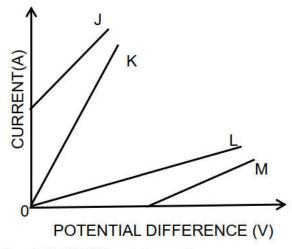
The resistor with the LARGEST resistance is . . .
