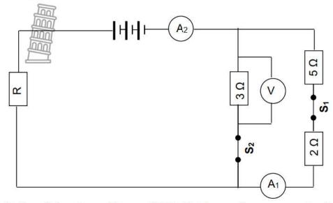
Both switches S<sub>1</sub> and S<sub>2</sub> are CLOSED. The reading on ammeter A<sub>1</sub> is 1,2 A.
